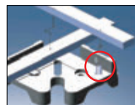
Use the provided leveling screw and optional Magnetic Rests to level long workpieces.
