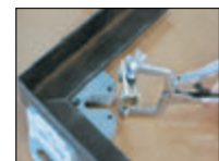
When the job is finished, easily slide the pliers out of the WP60 MagVise.
