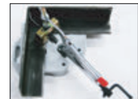
The pliers can mount from front side of the MagVise.
