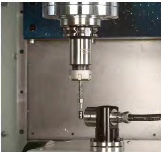
RENISHAW TS-27R AUTOMATIC TOOL LENGTH AND TOOL DIAMETER MEASURING DEVICE
