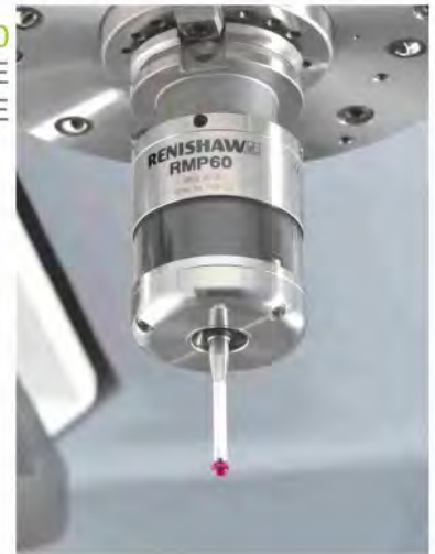
RENISHAW RMP-60 AUTOMATIC WORKPIECE CENTER MEASURING DEVICE
