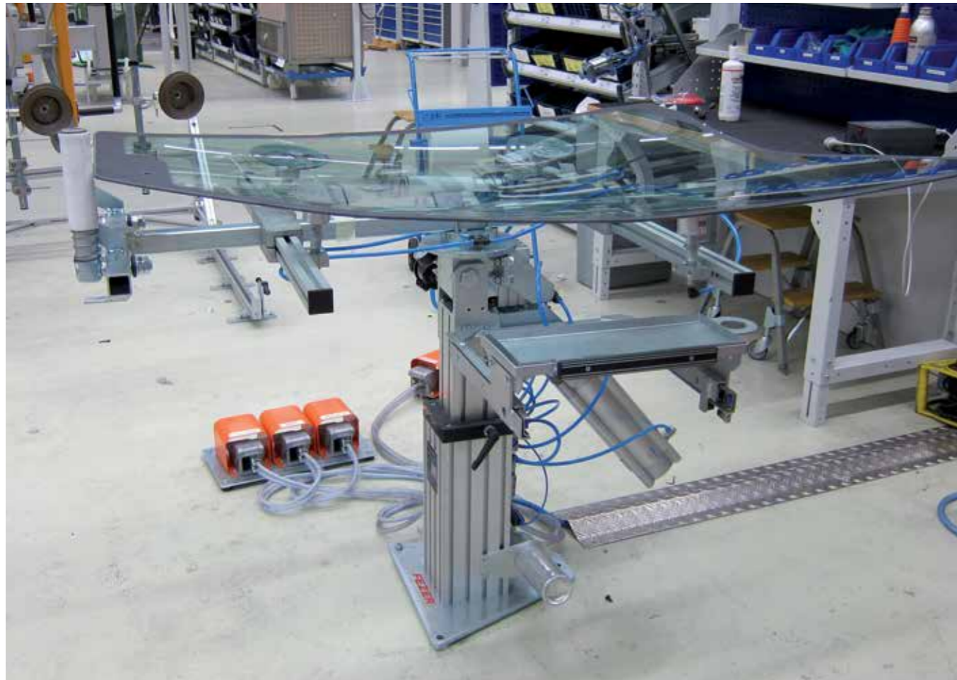
VacuStand VS-I with pneumatical swivel attachment for installation of side and back windows on cars
