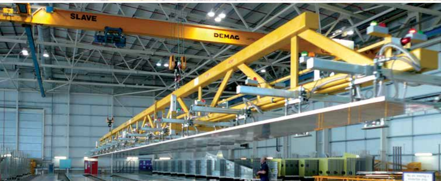
Transport of 36 m long aluminum sheets weighing 4.500 kg for the manufacture of wing parts for the Airbus A380
