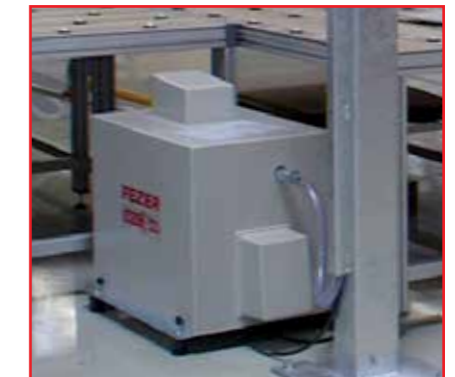
Silencer box to reduce the noise level
