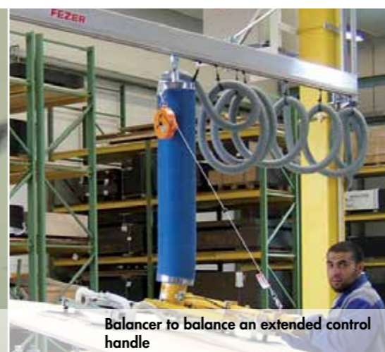
Balancer to balance an extended control handle
