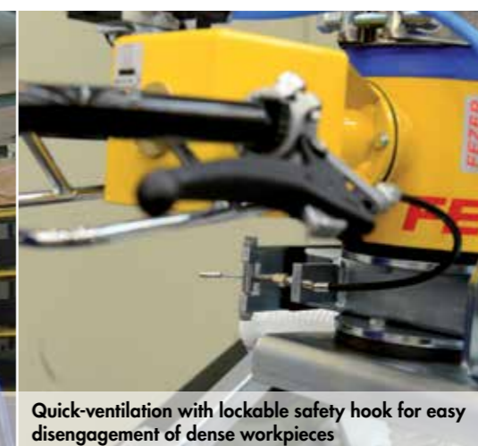
Quick-ventilation with lockable safety hook for easy disengagement of dense workpieces
