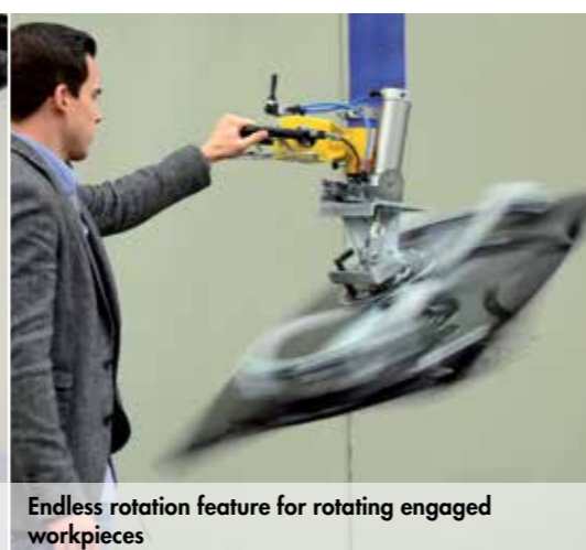
Endless rotation feature for rotating engaged workpieces
