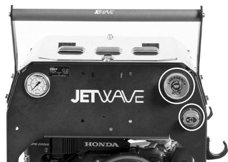
Figure.6 - Hornet G2 E-Stop & Battery Isolator
