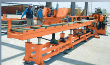
Tube 0506CO - Loading 5Ton, 6m
