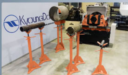
Tripod - Loading 0.5Ton
