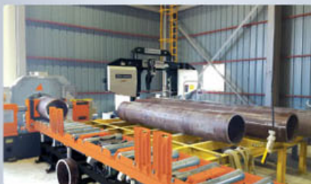
Cutting & Beveling line
