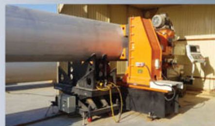
Hydraulic loading support - Loading 4Ton
