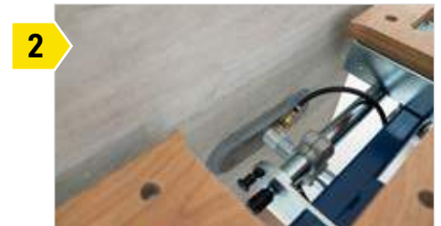
2 Vacuum clamping unit with two sliding oval grippers with touch valve.
