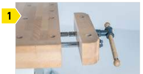
1 Workpieces can be clamped against the table with the help of the front gripper.
