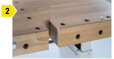
2 With the rear clamp, workpieces can also be clamped with bench hooks.
