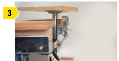
3 If necessary, the vacuum clamping unit can be folded away under the worktop.
