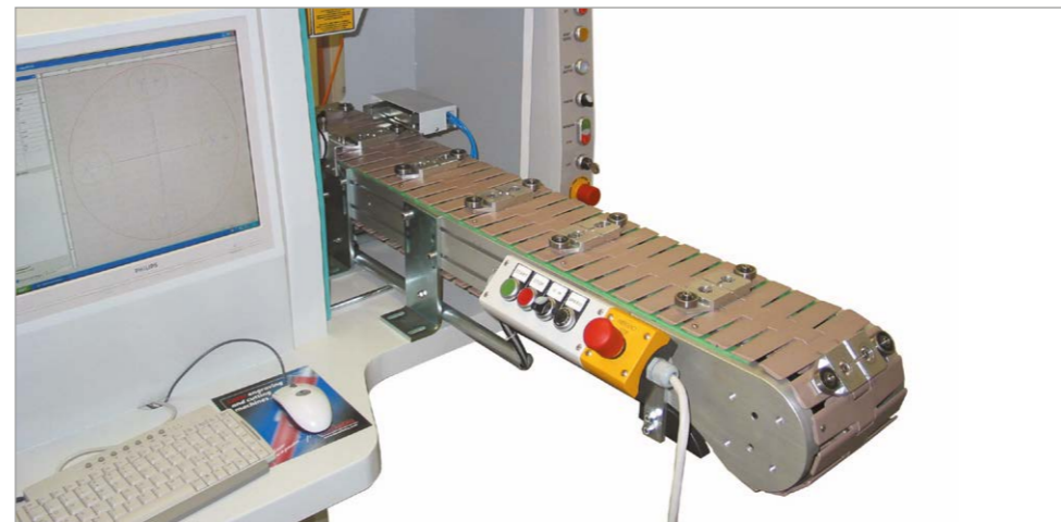
BELT A rotative belt servo device with indexing, for accurate positioning of piece holder tools. It allows the automatic release of the piece, leaving to the operator the only duty of ergonomic and safe loading.
