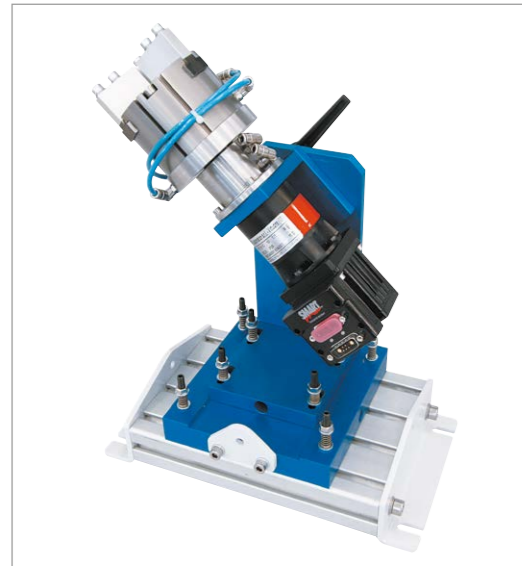
C PLUS AXIS Device for the round object engraving. Mounted on an anodised aluminium slideway, it has an 80 mm diameter self-centring chuck, with pneumatic collet opening through control lever.
