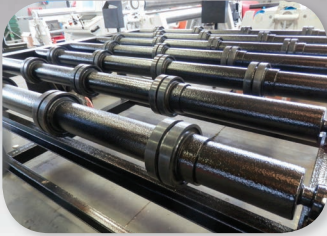
RUBBER COVERED CONVEYOR
