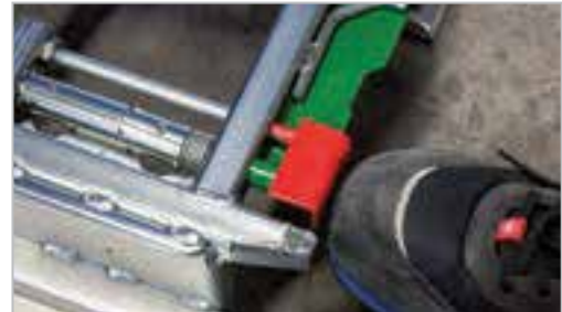
Easy lock/unlock mechanism with red and green foot pedal.
