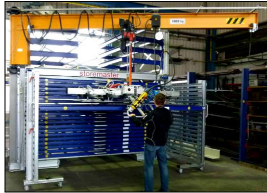
MasterTower ® TT with crane and vakuumlifter
