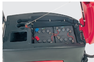
Machine open showing the batteries
