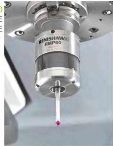
RENISHAW RMP-60 AUTOMATIC WORKPIECE CENTER MEASURING DEVICE
