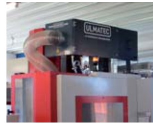
Oil mist separator installed on processing centre
