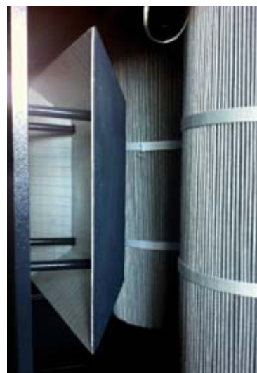
Ceramically coated pre-separator sheet for abrasive materials
