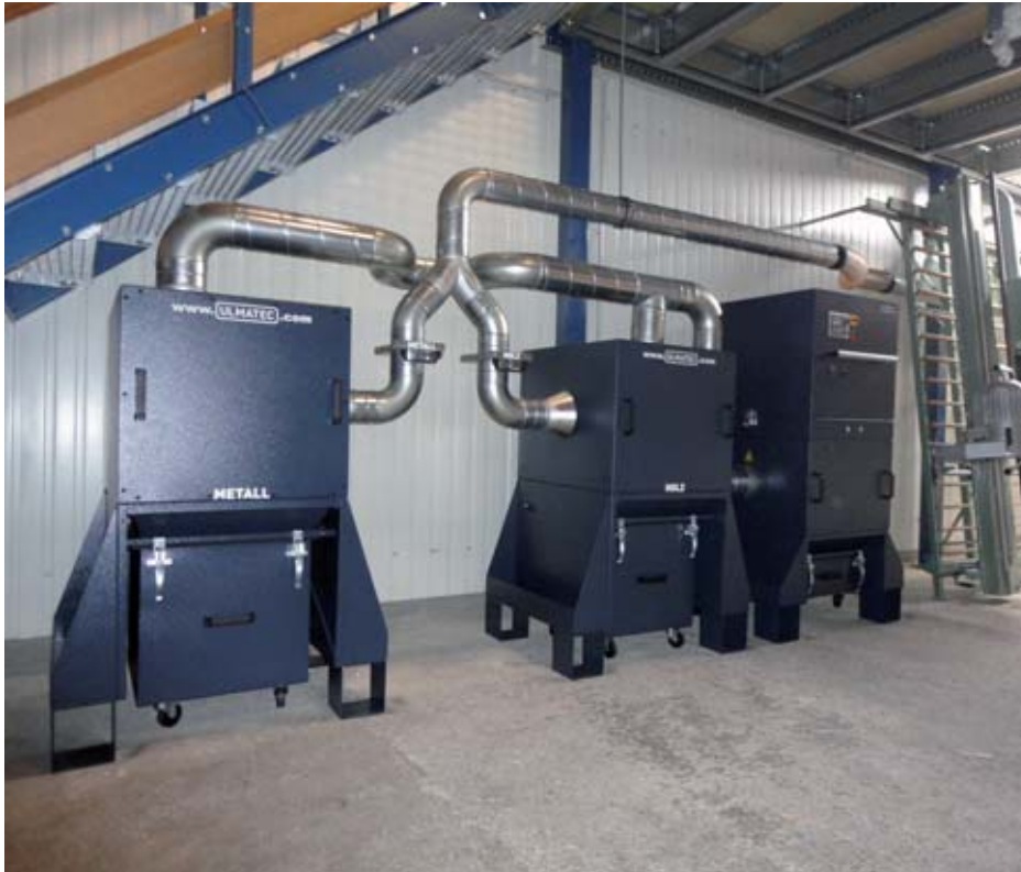
IEP 15-2-2 / 8.5 HD with baffle plate pre-separator (PVA)
