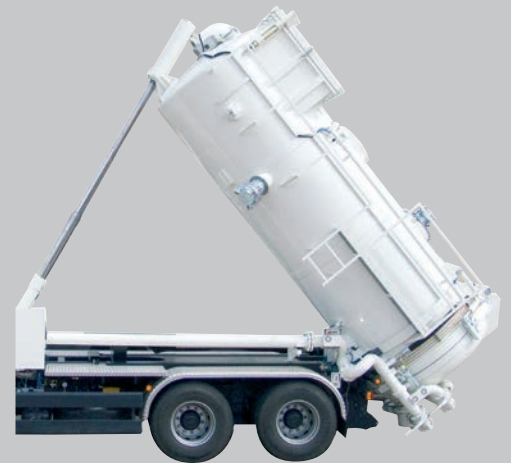
Hydraulic inclination of the collection container, tipping angle 60°
