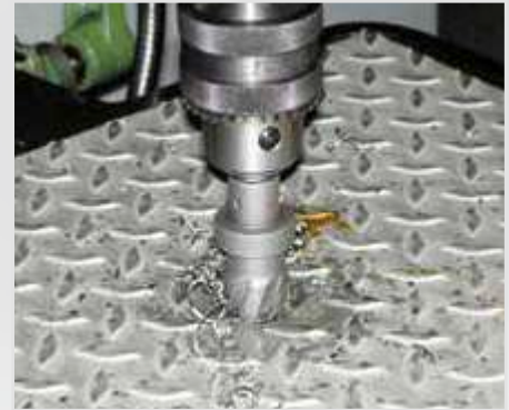
Drilling structured sheet metals
