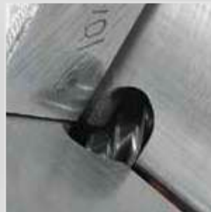
Precise deburring by rolling milling
