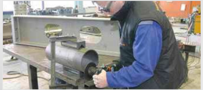
Start holes from \varnothing 20 mm.
