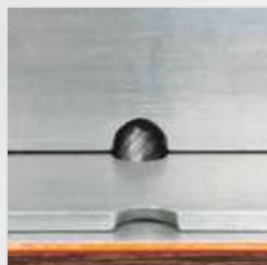
Position II: Material thickness from 1.5 mm
