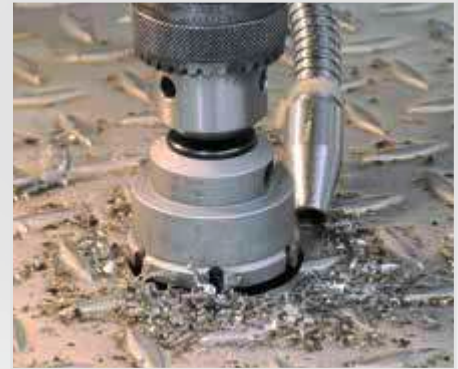
Drilling in checker sheet
