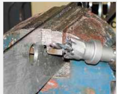
Free-hand drilling up to Ø 30 mm
