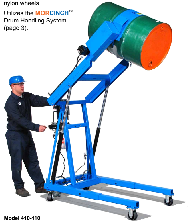
Model 410-110 • 72" (183 cm) maximum pour height • Electric power (AC 1-phase 115V) drum lift and tilt
